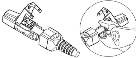
⑥ Close plug cover, make sure the drain wire is in proper contact with grounding clip on plug. Pull back strain relief boot to cover the plug, fasten supplied cable tie to secure grounding contact.
