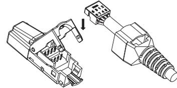
⑤ Place the wiring cap onto plug, use plier to clamp wiring cap until it completely snap-in to effect the connection.
